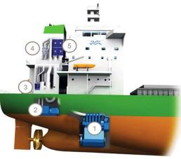
A waste-heat recovery system (WHRC) recover and use heat that is generated by existing vessel systems and otherwise lost. Heat can be collected from exhaust gases, excess steam, or cooling water and used to generate electricity on board, typically for auxiliary engines that would otherwise rely on marine diesel fuel.
